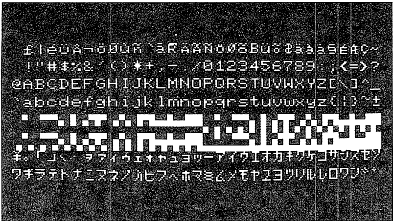
Fig. 1-6. Character set available with bit 3 port ECH low on TRS-80 Model III.
